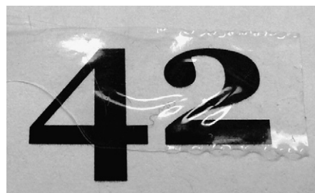
Fig. 5. Photograph of a P-R-HBA- l -PDMS 5,6 conetwork with a PDMS content of 49 wt%.
